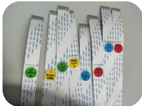
6.10 Data line: 14 core flat line of the nozzle and head plate, one nozzle needs 4
